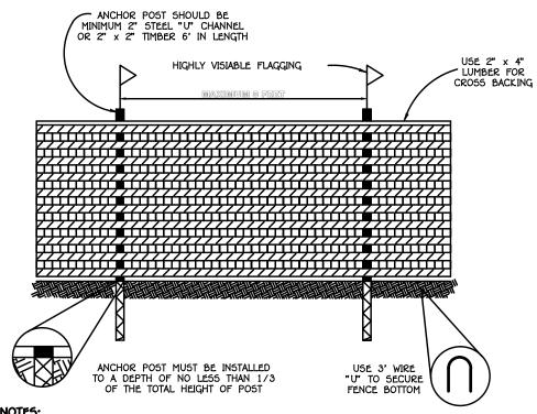
RETENTION AREA WILL BE SET AS PART OF THE REVIEW PROCESS. BOUNDARIES OF RETENTION AREA SHOULD BE STAKED AND FLAGGED PRIOR TO INSTALLING DEVICE. ROOT DAMAGE SHOULD BE AVOIDED. PROTECTIVE SIGNAGE MAY ALSO BE USED
