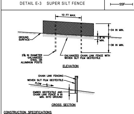
INSTALL 2% INCH DIAMETER GALVANIZED STEEL POSTS OF 0.095 INCH WALL THICKNESS AND SIX FOO LENGTH SPACED NO FURTHER THAN 10 FEET APART. DRIVE THE POSTS A MINIMUM OF 36 INCHES INTO THE GROUND.
