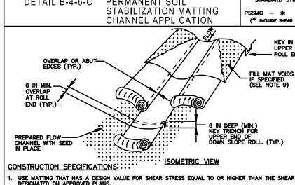
USE MATTING THAT HAS A DESIGN VALUE FOR SHEAR STRESS EQUAL TO OR HIGHER THAN THE SHEAR ST DESIGNATED ON APPROVED PLANS.
